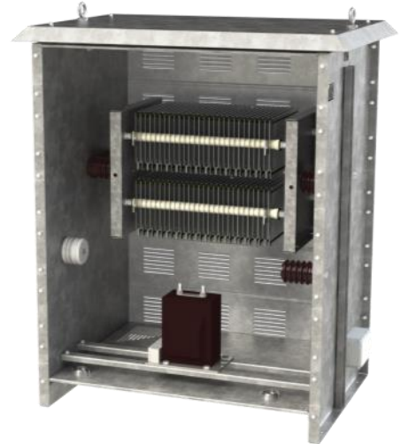
IP23 resistor: 75 Ohm. 50 Amp. - 10 sec. Insulation Level: 12 kV.
